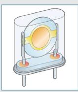
reproducibility and lower sensitivity to contamination than other available trace moisture analyzers. Water molecules are adsorbed into the moisture sensitive layer deposited on the crystal surface and the resulting change in mass modifies, in a very precise and repeatable manner, the frequency of oscillation. The design and manufacturing quality of the Michell QCM sensor is the key to the high
